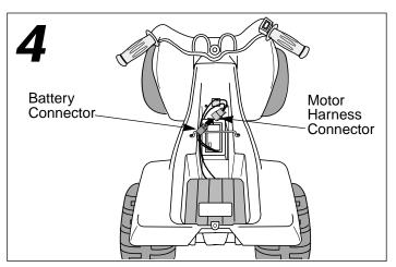
• Plug the battery connector into the motor harness connector.
